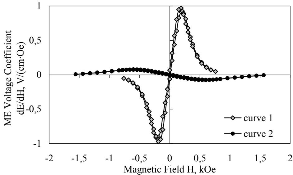
Figure 1. Field dependence of longitudinal and transverse ME voltage coefficients for trilayer structure of permendur-PZT-permendur.
