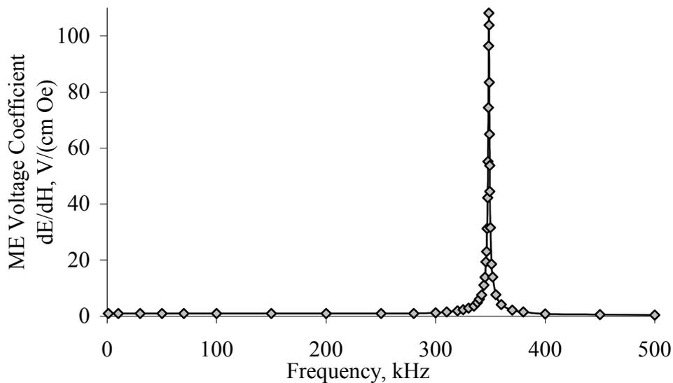
Figure 2. Frequency dependence of ME voltage coefficient for trilayer structure. The bias field  $H$  was set for maximum ME coupling.
