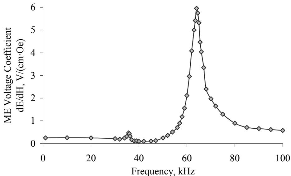
Figure 3. Frequency dependence of ME voltage coefficient for bilayer structure. The bias field H was set for maximum ME coupling.
