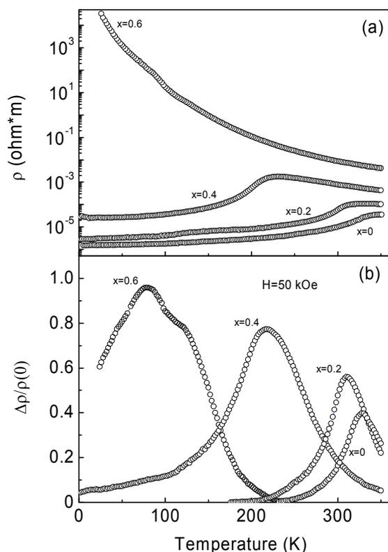
Fig. 1. (a) Temperature dependencies of the resistivity  $\rho$  and (b) magnetoresistance  $\Delta\rho/\rho(0)$  for  $(\text{La}_{1-y}\text{Eu}_y)_{0.7}\text{Pb}_{0.3}\text{MnO}_3$  crystals.
