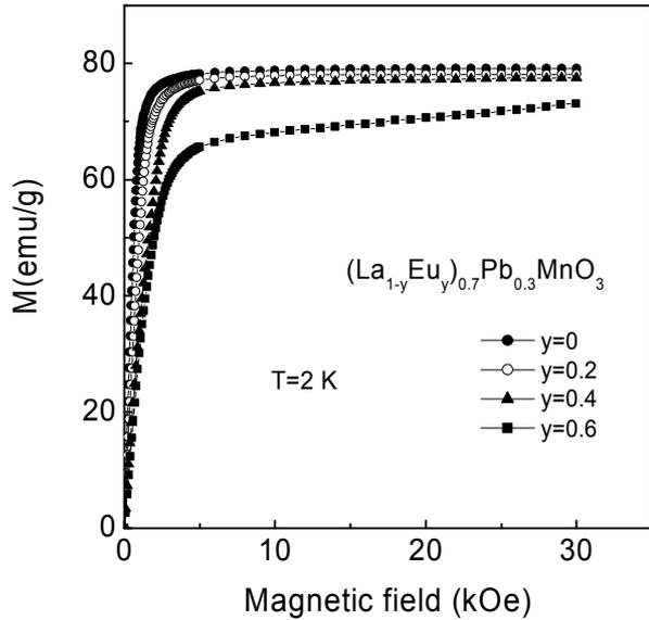
Fig. 2. Magnetic field dependencies of the magnetization for  $(\text{La}_{1-y}\text{Eu}_y)_{0.7}\text{Pb}_{0.3}\text{MnO}_3$  crystals.
