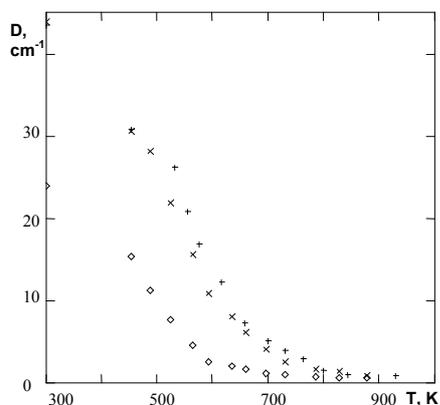
Fig. 1 Intensity of the  $\sim 36000 \text{ cm}^{-1}$  absorption band as function of annealing temperature for  $\text{Gd}_3\text{Ga}_5\text{O}_{12}$  irradiated with fast neutrons:  $\times$  – annealed in electric field;  $+$  – annealed without field; and  $\text{Gd}_3\text{Ga}_5\text{O}_{12}:\text{Ca}$ :  $\diamond$  – annealed without field.
