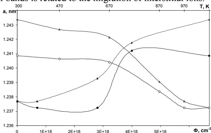
Fig. 2. Lattice parameter of  $\text{Gd}_3\text{Ga}_5\text{O}_{12}$  as a function of neutron fluence:  $\bullet$  – fast neutrons,  $\blacktriangle$  – thermal neutrons. Lattice parameter of  $\text{Gd}_3\text{Ga}_5\text{O}_{12}$  as a function of annealing temperature:  $\circ$  – fast neutrons,  $\triangle$  – thermal neutrons.
