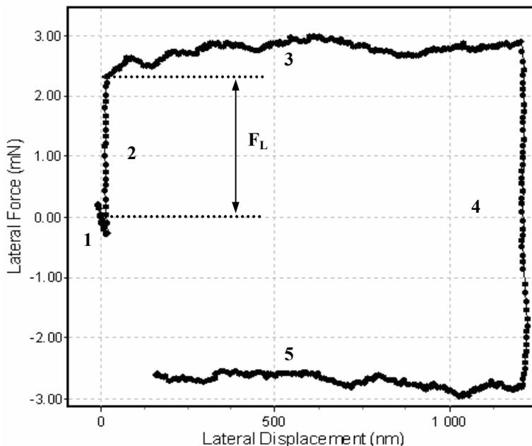
Fig. 2. Lateral force – displacement curve. The numeration of the parts of curves corresponds to the
