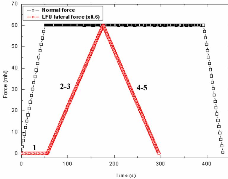
Fig.1. UMIS normal (the black line) and LFU lateral (the red line) force cycles. The normal force increases linearly within 55s up to the maximal value of 60mN (1). When the maximal value of the normal force is achieved the LFU lateral force is immediately started by hand. The LFU lateral force increases within 120s linearly up to 100mN (2-3) and decreases within 120s linearly to zero (4-5).
