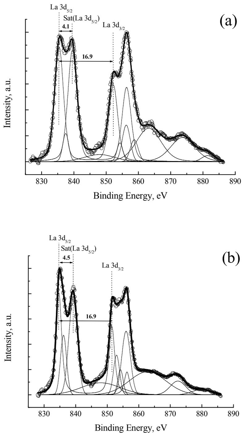
Figure 1. Deconvolution analysis of La 3d and Ni 2p signal of  $\text{LaNiO}_{3-x}$  thin films. (a) – “As grown”;(b) –  $\text{Ar}^+$  etched film. The scattered points refer to the raw data, the thin solid lines correspond to the spectral components and thick line is the spectra envelope.
